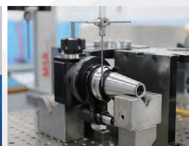
Circular sunout: \leq 20\mu\text{m} Angularity: \pm 8\mu\text{m}
