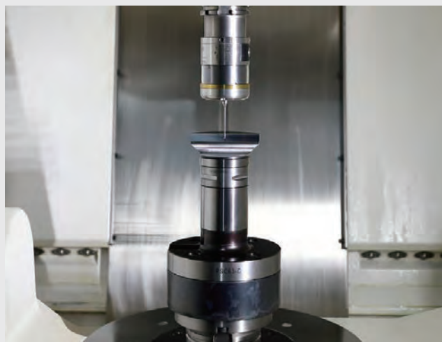
Setting rotary table machining origin of 5 axis machining centers
