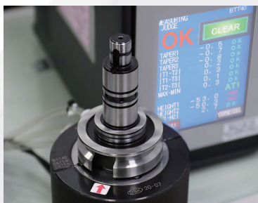
Taper tolerance: <AT3
