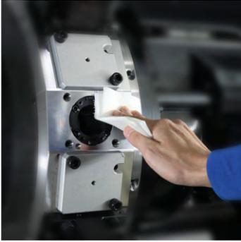
Clean the inner hole and end face of the turret with wiping paper.
