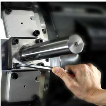
Mount the BMT turret master bar into the turret and tighten four screws with a L-shaped wrench.
