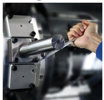
Use the L-shaped wrench to loosen the four screws of the BMT turret master bar.
