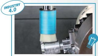
It can process the material hardness up to HRC52 and materials, e. g. aluminum, copper, metals, nickel alloy and alloy steel.
