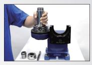
3. Install the collet chuck onto the assembly device.
