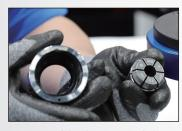
Disassemble the nut and the collet for cleaning and maintenance as well.
