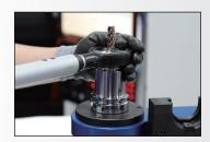
Install the collet chuck onto the assembly device, and use the digital torque wrench to loosen the nut in an anticlockwise direction.
