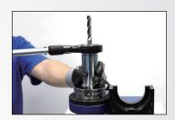
6. Use a torque wrench to fasten the nut evenly in a clockwise direction.
