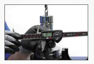
After inserting the tool, use a caliper to measure the length required.
