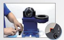
1. Install the collet chuck onto the assembly device.
