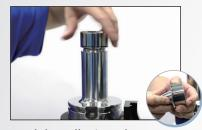
4. Load the collet into the nut, and assemble them with the collet chuck.
