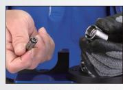
4. Disassemble the nut and the collet for cleaning and maintenance as well.
