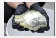
2. Put the tool holder into the anti-rust bag.
