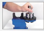
3. Install the tool holder onto the assembly device.
