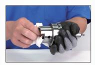
Use wiping paper to clean off the fluid on the tool holder surface.
