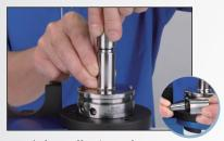
4. Load the collet into the nut, and assemble them with tool holder.
