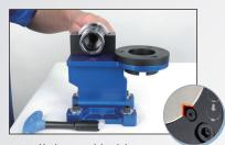
1. Install the tool holder onto the assembly device.
