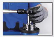
6. Use a torque wrench to fasten the nut evenly in a clockwise direction.
