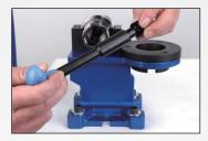
2. Use a key to fasten the coolant supply unit into the tool holder.
