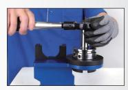
3. Install the tool holder onto the assembly device, and use the digital torque wrench to loosen the nut in an anticlockwise direction.
