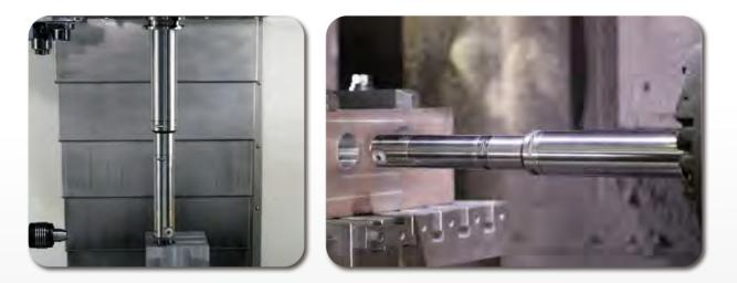
Silent Damping Genius equipped with damping mechanism eliminates vibration, improves workpiece surface finish, roundness, tool life, maintains spindle precision, and increases the overall production efficiency!
