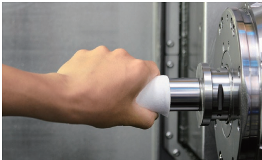
After loading the spindle mater bar into spindle, wipe down the straight shank.
