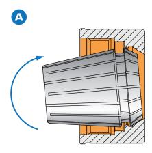
Put the collet in the clamping nut. Let its collet taper contact the spring ring well. Toward the arrow direction, push slightly, and then you can put it in.
