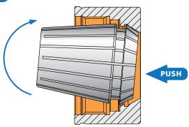
Loosen the nut from the body, and then take out the end mill. Toward the arrow direction, push slightly, and then the collet can be taken out.
