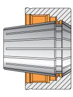
Insert the end mill (cutter) into the body. Tighten clamping nut by wrench. Then it is ready for operation. (Do not tighten the clamping nut before the cutter is installed.)
