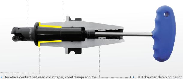
Two-face contact between collet taper, collet flange and the end of HBL tool holder, increases the rigidity of machining.
