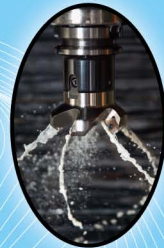
Cutter with coolant holes design:
